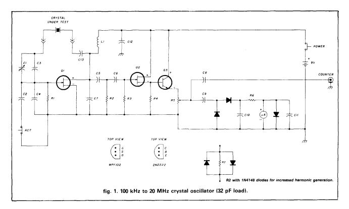
counter output is tied to the wiper of the pot but could also be connected directly to the emitter of Q3, if desired.
